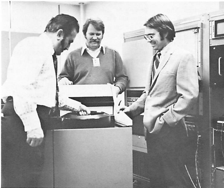
Al Hasler places a Memorex Disc Pack on the new 3675 Disc Module during a thermal expansion test which analyses temperature effects on the drive's operation, while Ron Higgins and Robert Temporo look on. Dave Reech (not pictured), has recently been promoted to Mechanical Engineer II and is now a member of this team.
