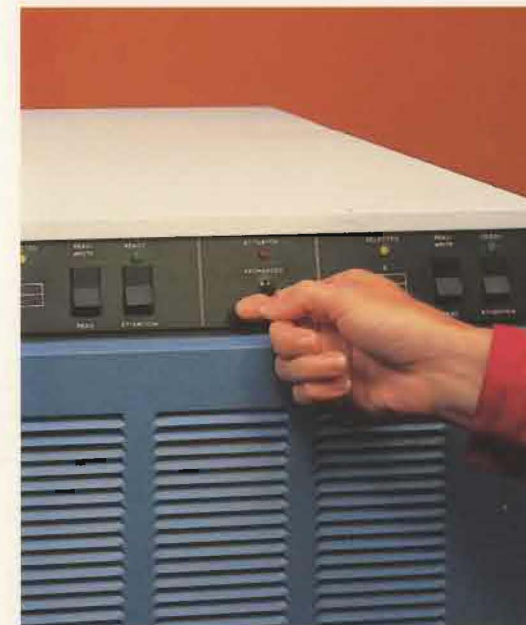
The 3680's standard actuator electronics switch feature improves the data availability of the disc subsystem. In the event that a malfunction in the logic should occur, the actuator electronics switch enables the read/write logic associated with one actuator in a spindle to be switched to the other actuator without changing the original actuator's address.
