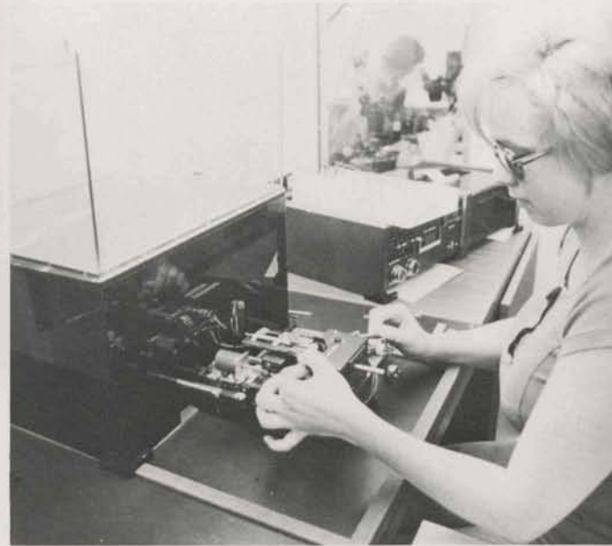
Figure 2. Memorex designed tester measures read/write head "flying heights" of ten microinches.
