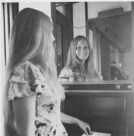
Pretty Donna Paoletti demonstrates the new "Videoguard" system. In photos (left to right), she enters the booth, places her badge in the pocket and looks toward the mirror, and her picture is displayed on the closed circuit TV screen for identification by the officer.
