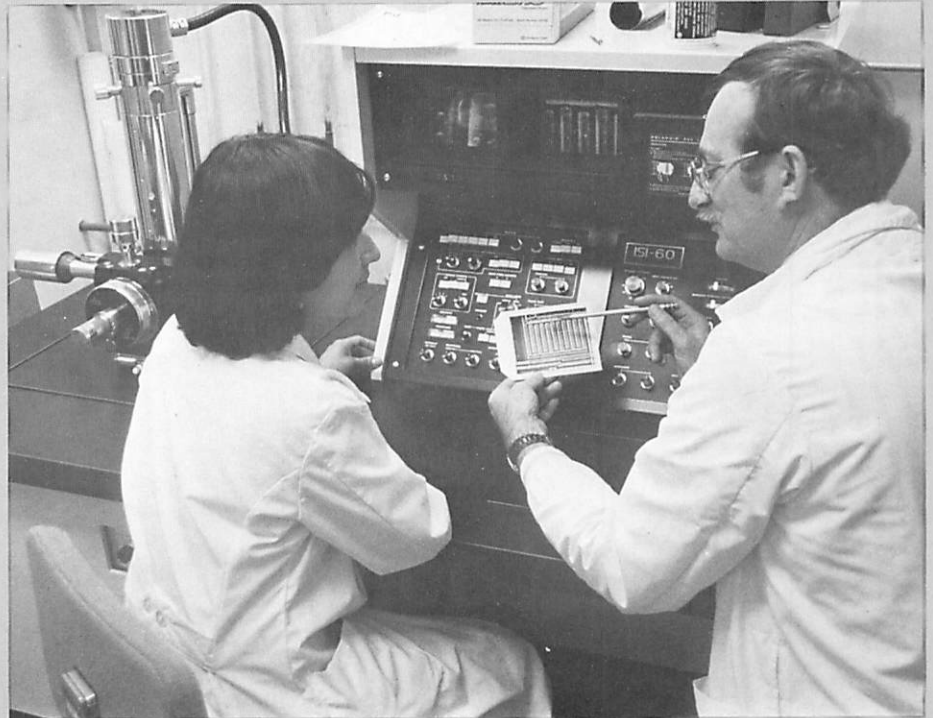
Garry Johnson shows Dora Devilliers photo of defective integrated circuit taken with new scanning electron microscope.
